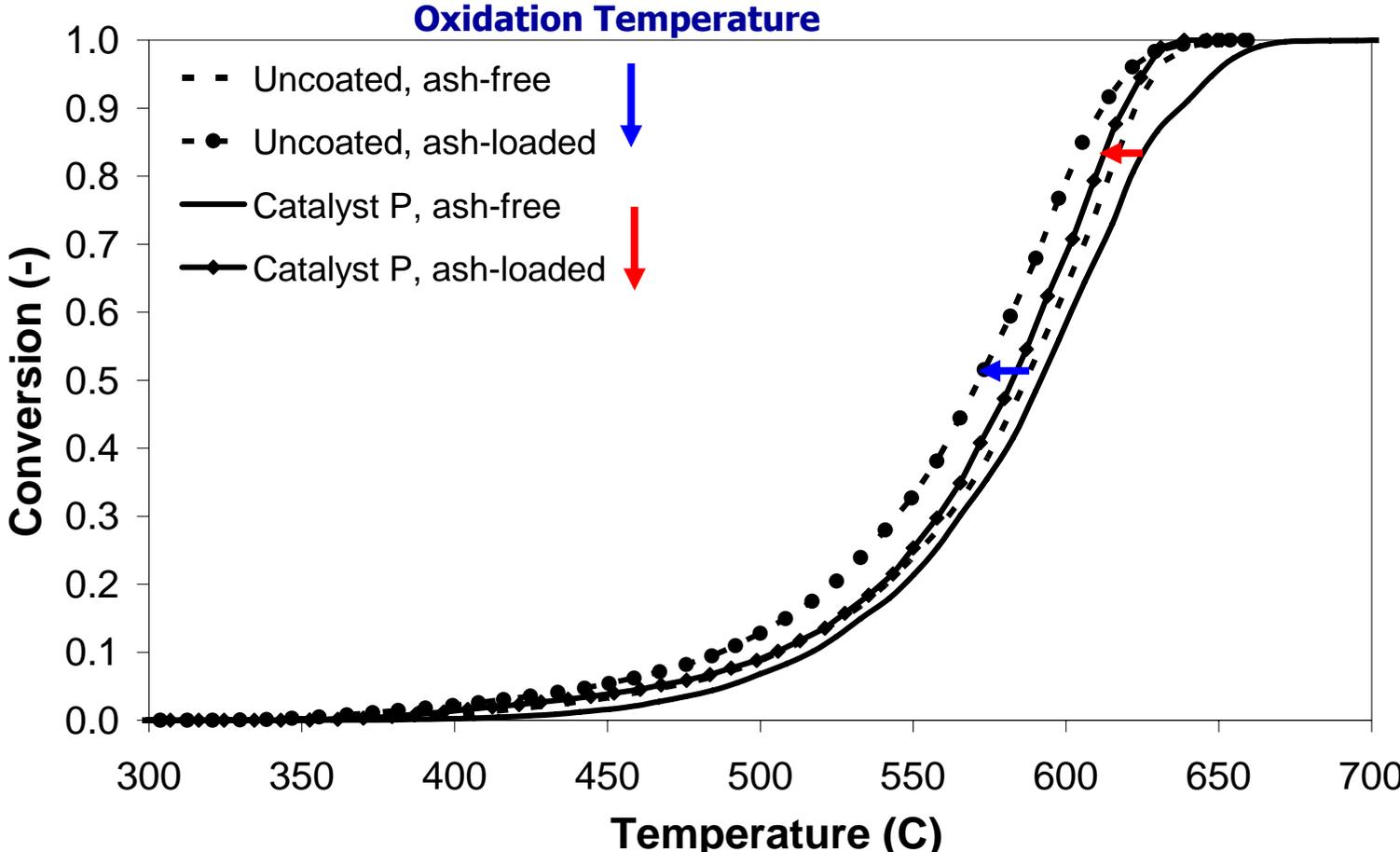
Small shift of the soot conversion curve to lower temperatures due to ash accumulation for both the uncoated filter and **Catalyst P**.
