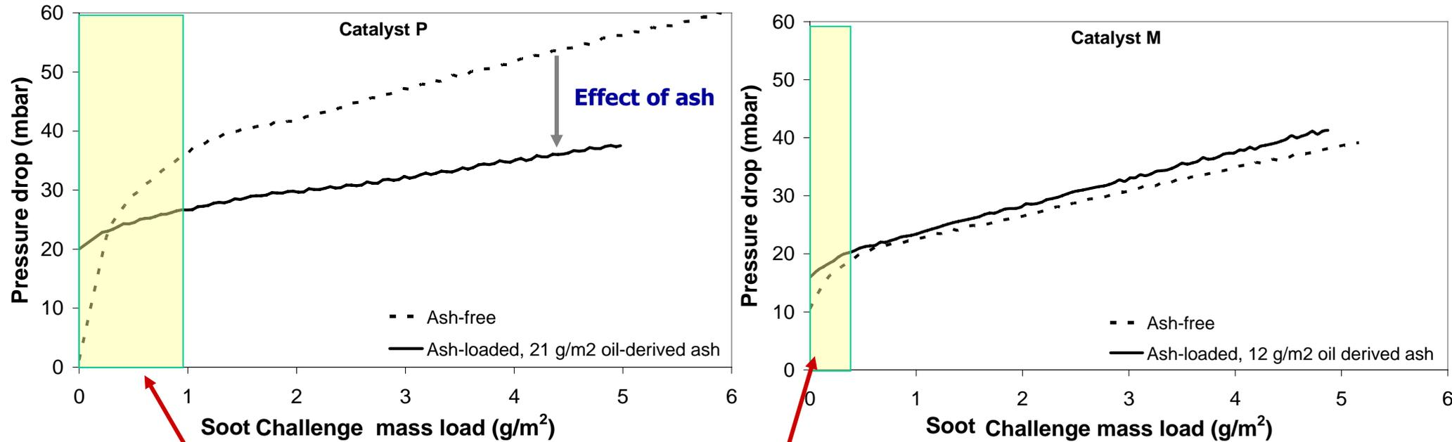
The existence and extent of the deep bed filtration regime (irrespective of whether the filter is coated or uncoated) determines how the accumulating ash layer impacts the filter pressure drop during soot loading.
