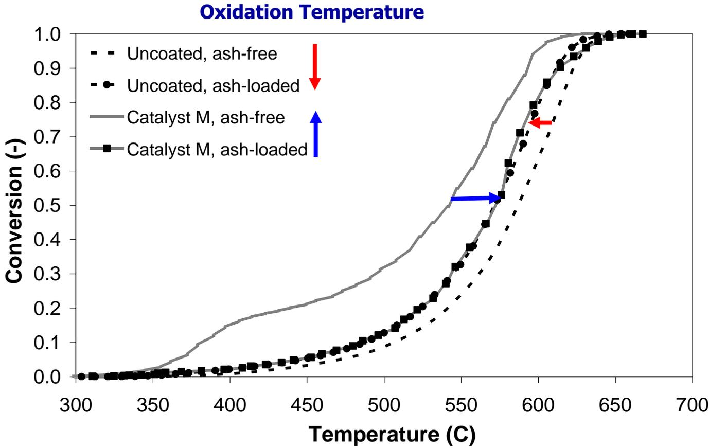
**Significant loss of the catalytic activity of Catalyst M due to ash. The ash-loaded catalyzed filter oxidizes soot like the uncoated ash-loaded filter.**
