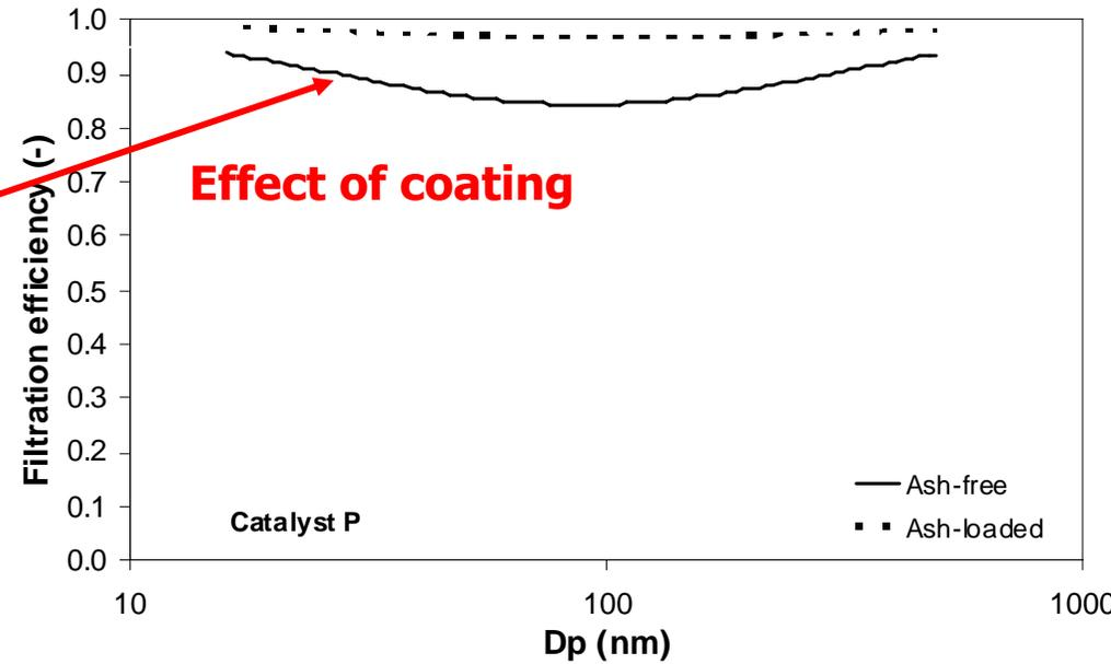
**Significant increase in the filtration efficiency due to ash particle accumulation for both the uncoated and the catalyzed filter.**
