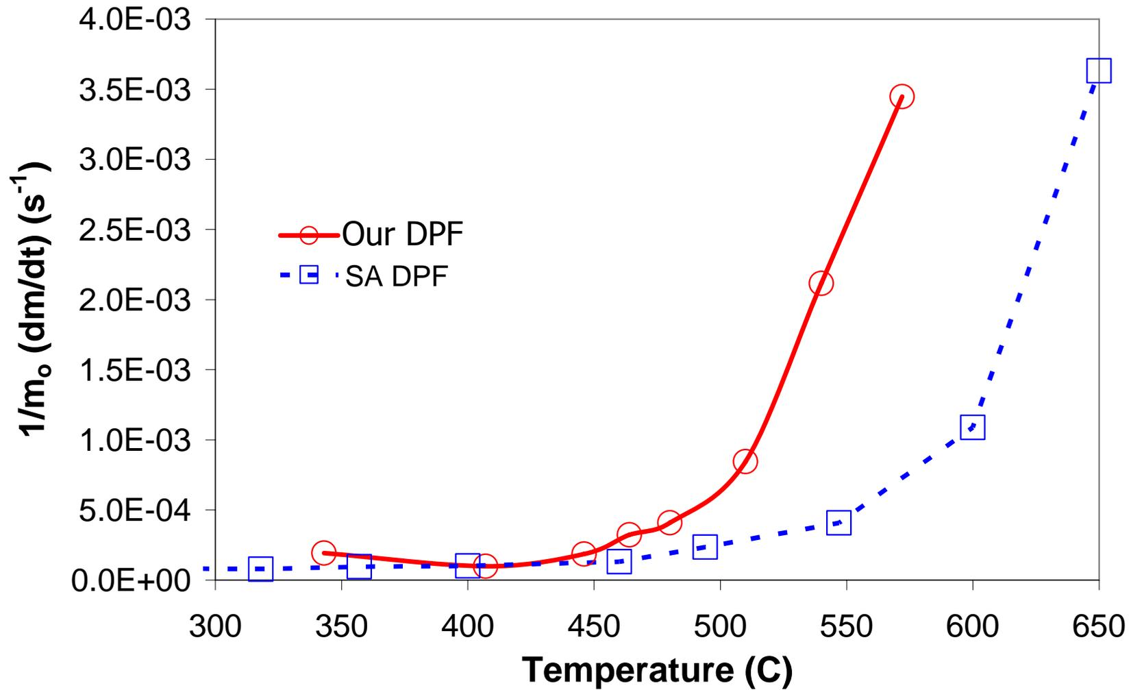
4 times higher soot oxidation rate at 550 C compared to the SA DPF.
