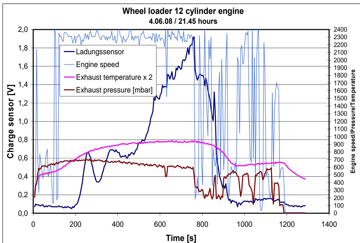
During this procedure the emission rises by factor 19 from 0,1 [V] up to 1,9 [V].
