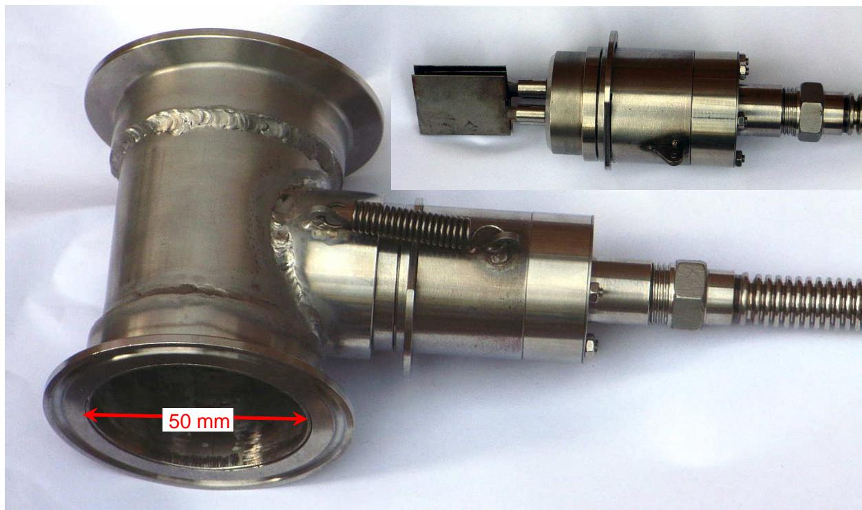
In heavy duty machinery and non road applications it is mostly not possible to get the necessary information for calculating the exhaust-gas speed. In this case specific engine operating points are used for measuring a calibrated smoke emission, like full-load condition. For identifying this operation mode the engine speed, derived from the generator impulses, and the exhaust gas temperature are measured.
