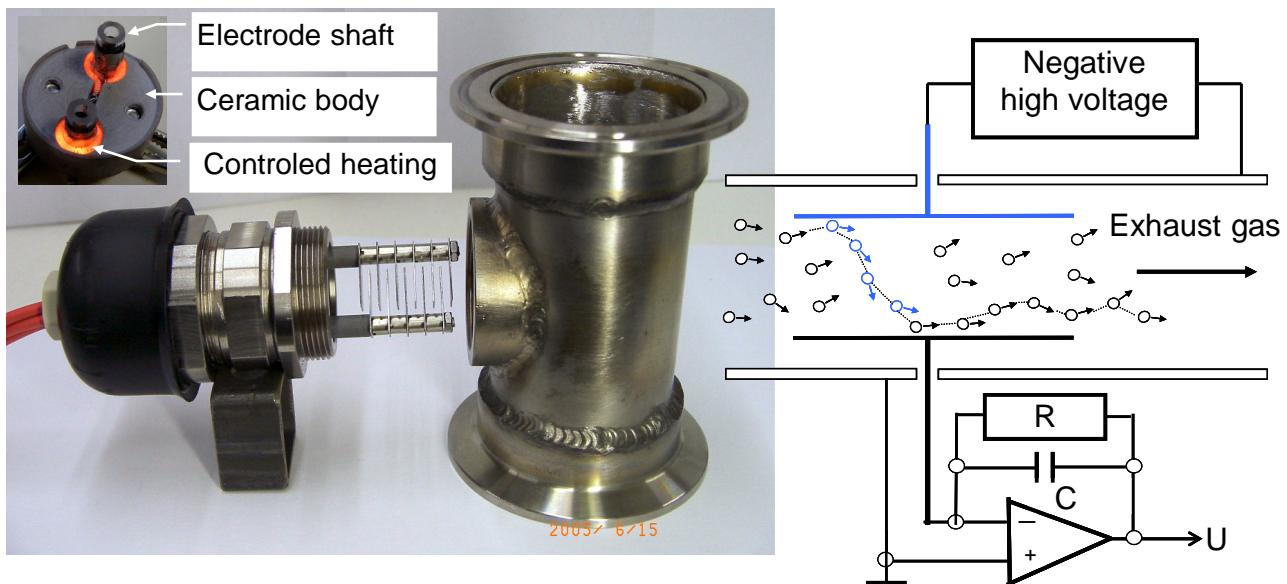
Soot particles are attracted by Coulomb forces on to the high voltage plate and receive there a strong charge whilst touching it. As the polarity is equal the particles are repelled on to the virtually grounded plate. The DC- coupled charge amplifier measures the charge of the particles they have transported.
