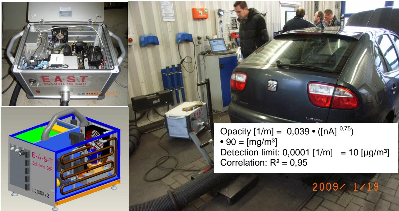
Further applications of the soot charging sensor for test bench investigations of the quality of diesel combustion processes are shown in next diagram.
