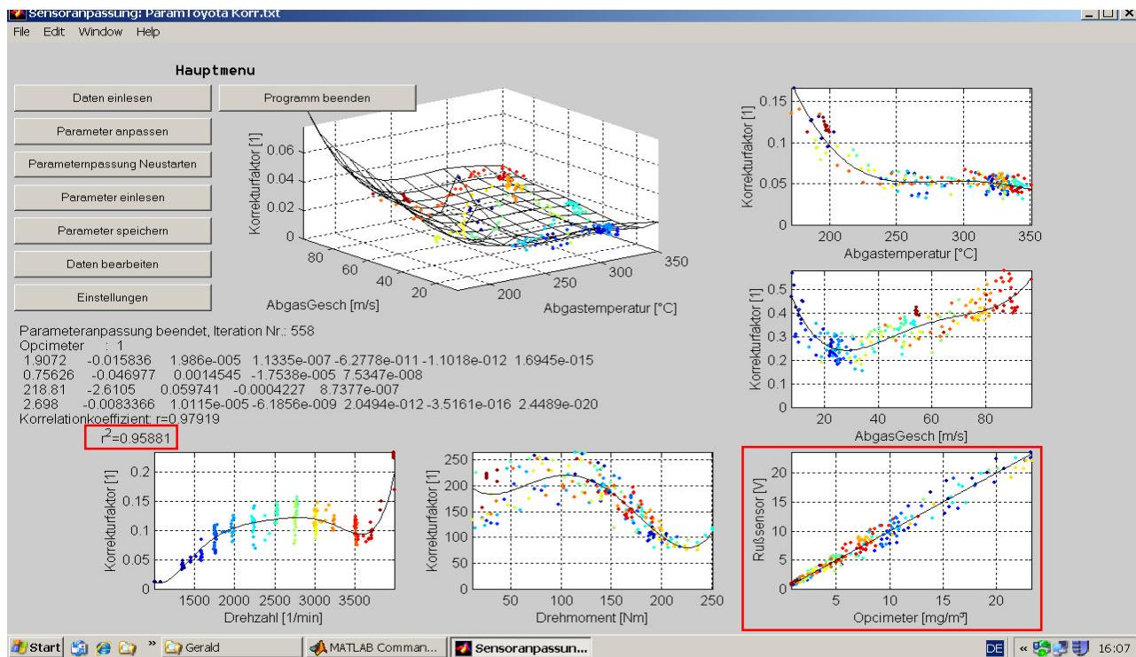
Chosen parameters which have influence on the quality of the soot particles are measured across the complete engine map. In this case engine speed, exhaust gas temperature, torque and the exhaust gas speed are chosen. Instead of torque and exhaust gas speed
