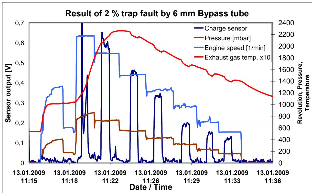
The result shows that a trap fault of 2 % can be detected even at no-load operation of the engine under OBD conditions.
