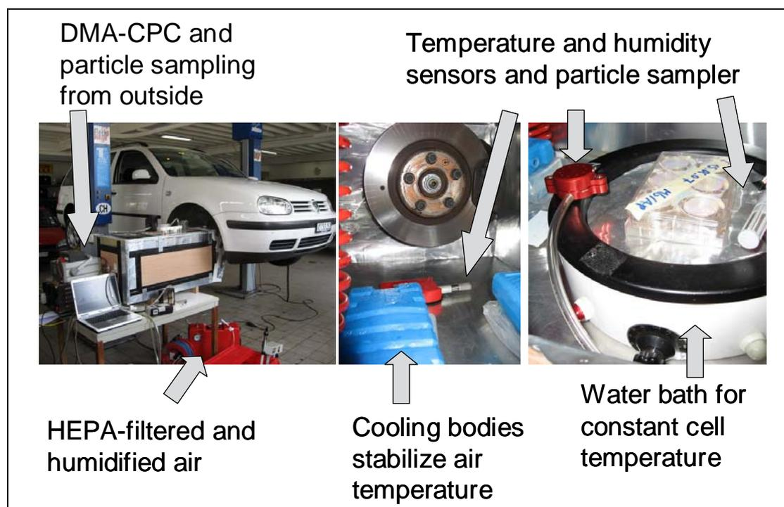
**Figure 1:** *Left:* Exterior view of the exposure box with particle measurement equipment (Grimm DMA-CPC, particle sampling pumps) and pump and humidification system for air preparation. *Middle:* View onto the brake disc with sensor placement and cooling bodies to stabilize air. *Right:* A water bath was used to maintain stable cell culture temperature.
