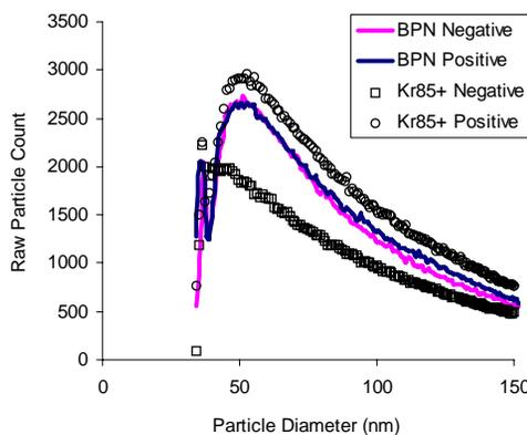
Fig. 2: Size Distributions as measured using the radioactive and electrical neutralizers with the DMA scanning both positive and negative high voltages.
