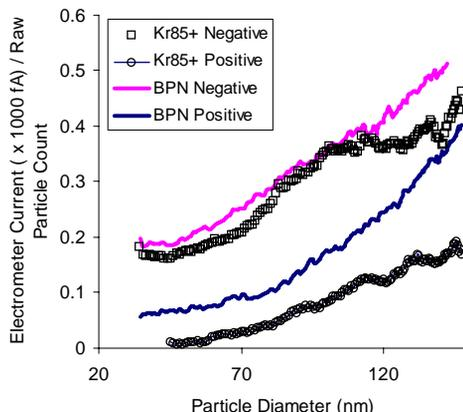
Fig. 3: Comparison of charge per particle vs particle diameter for the Kr85+ source and the BPN.
