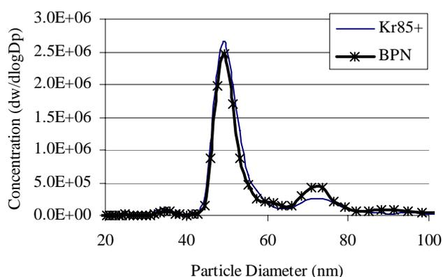
Figure 2 Example size distributions measured when passing a mono-disperse aerosol (50 nm) through either a radioactive ( $\text{Kr}^{85+}$ ) or electrical neutralizer.
