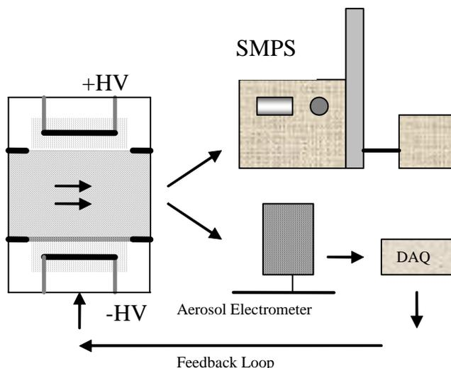
Fig. 1: Typical setup of the BPN. The aerosol passes through the bi-polar charging region after which the flow is directed to an aerosol electrometer and a chosen measurement instrument.
