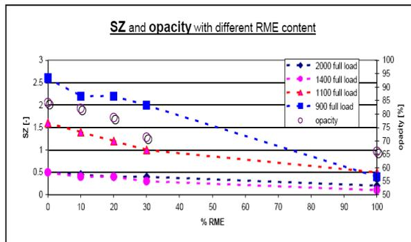
This was explained by coulometric analysis which showed a reduction of elemental carbon EC when increasing the RME content. Size distribution analysis proved that the number concentration of particles above 60 nm mobility size was reduced, the number concentration of particles smaller than 60 nm however was rather increased.
