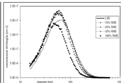
The size distributions in the size range 15 – 600 nm (mobility diameter) were analyzed for all blending ratios and at all operating points. The examples show the size distribution for full-load and 25% load at medium RPM. The data confirms the published effect [1] The blending of RME noticeably diminishes, and pure 100% RME clearly curtails the number of the large particles. However, all tests reveal that RME blended fuel tend to increase the count of finer particles.
