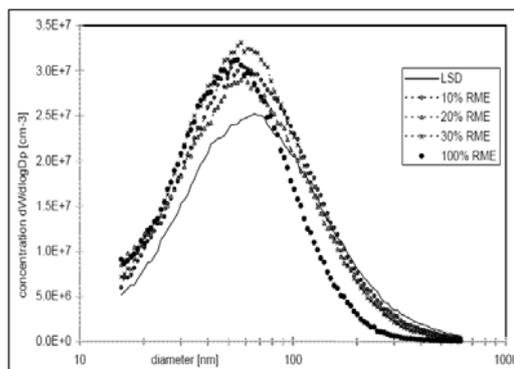
Filtration efficiency was about equal for all blends (> 99 % for all size classes 20 – 300 nm) and regeneration characteristics did not show any significant difference with the different fuels. With respect to other pollutants there was again no significant influence neither for NOx, CO and HC nor for particle bound PAH.
