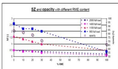
Due to its favorable O<sub>2</sub>/C ratio, RME the share of EC. The smoke metric (SZ) and the opacity during free acceleration confirm this very distinctive trend.
