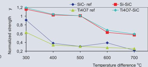
Figure 10. Normalized fracture strength of DPF material after thermal shock loading.
