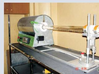
Figure 8. Thermal shock test bench.
