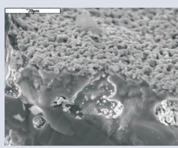
Figure 4. SEM image of  $Ti_4O_7$  sphere bonded to SiC.
