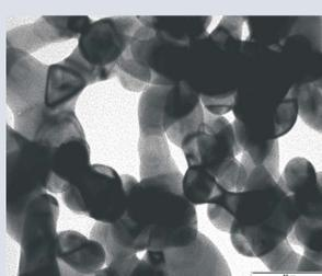
Figure 7. SEM image of PdRu<sub>3</sub> deposited on high porosity  $Ti_4O_7$ -SiC.
