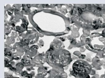
Figure 5. TEM shows a micro-section of  $Ti_4O_7$  nanosphere sinters by PPS method.
