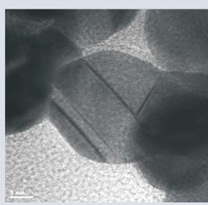
Figure 3. HRTEM shows the crystal defects of flame generated  $Ti_4O_7$  sphere.
