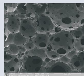
Figure 2. SEM image of high porosity- macro- and mezo-pores  $Ti_4O_7$  foam filter-ref.
