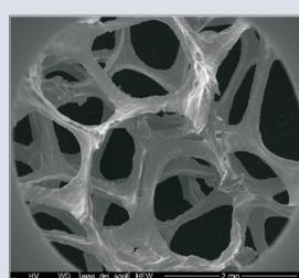
Figure 6. SEM image of porosity of PdRu<sub>3</sub>-sinter.
