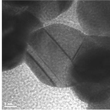
Figure 1. HRTEM shows the crystal defects of flame generated  $Ti_4O_7$  sphere.
