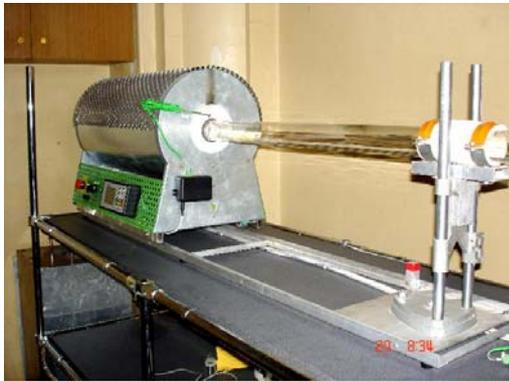
Figure 2. Thermal shock test bench.
