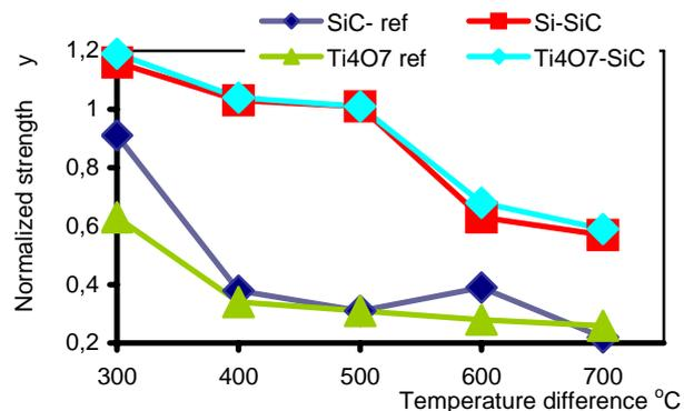
Figure 3. Normalized fracture strength of DPF material after thermal shock loading.
