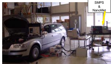
Test vehicle and measuring systems for nanoparticles analysis on a chassis dynamometer
