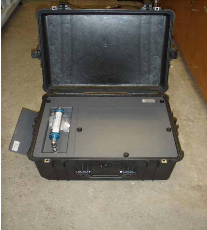
Measures real-time mass emissions (PM, NO<sub>x</sub> in g/sec and g/km plus opacity) from vehicle in motion
