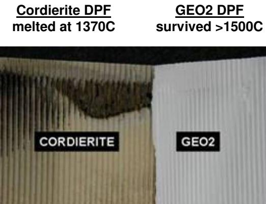
**Thermal Cycling, fatigue testing ongoing**
