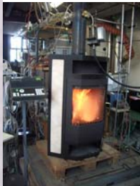
Pic 1: Picture of the wood stove used for the experiment. The wood stove has a small combustion chamber (volume: 0.06 m 3 ) lined with fireclay and no "after burning chamber".
