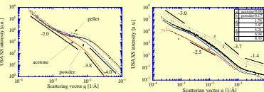
Left: SAXS scattering curves for diesel soot as powder, pressed pellet, and immersed in acetone. Sample environment influences soot aggregation slightly and has impact on scattering curve. Right: Shift of characteristic structures in scattering curves upon pressurizing of samples indicates aggregate rearrangement.
