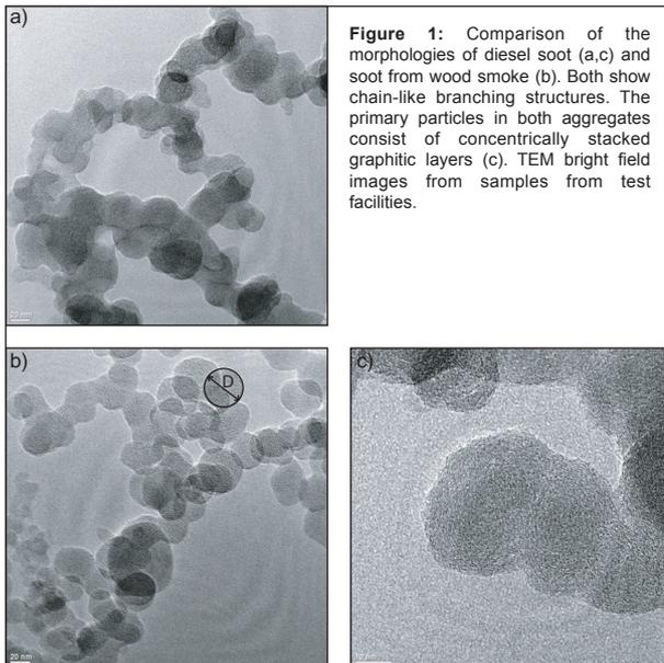
**Figure 1:** Comparison of the morphologies of diesel soot (a,c) and soot from wood smoke (b). Both show chain-like branching structures. The primary particles in both aggregates consist of concentrically stacked graphitic layers (c). TEM bright field images from samples from test facilities.
