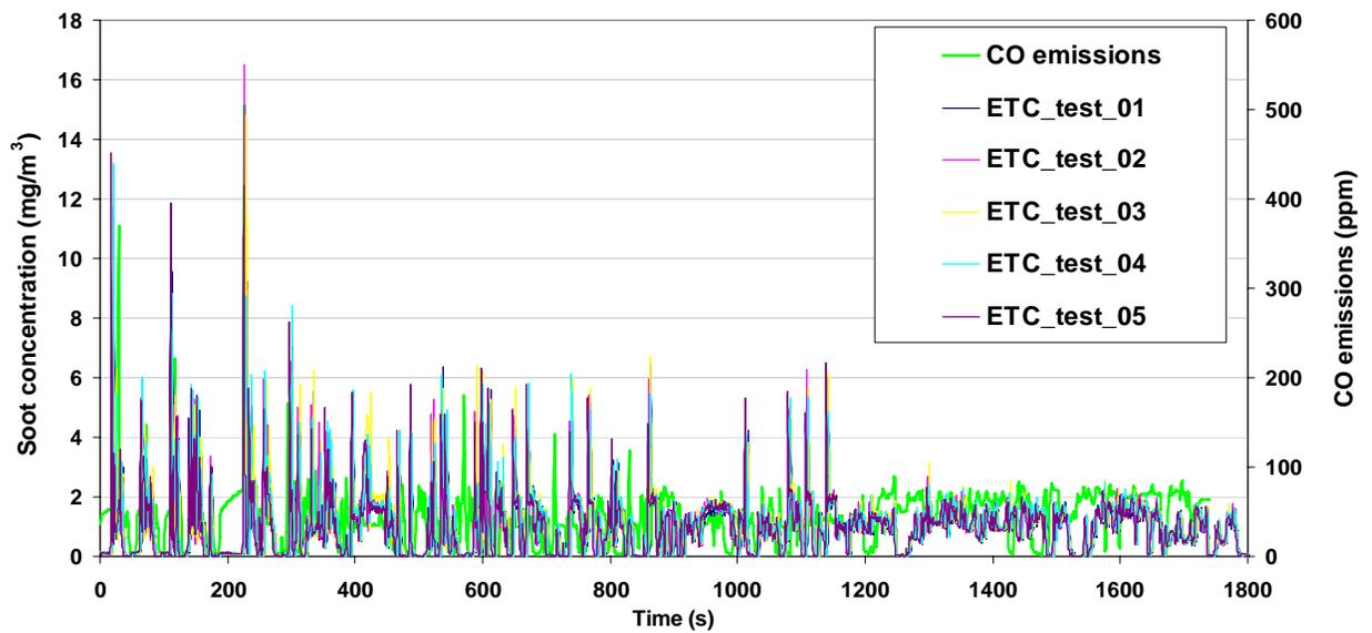
**Figure 4:** AVL 483 MSS data vs. test time for 5 consecutive ETC tests; CO emissions on the right-hand axis.
