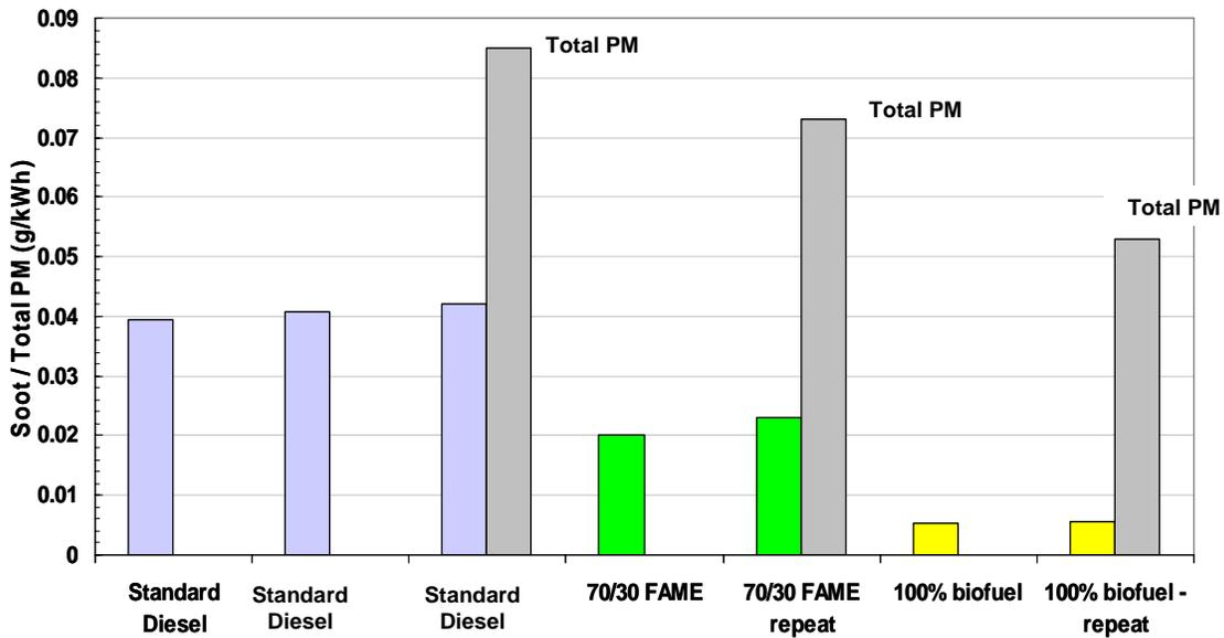
**Figure 6:** Total PM mass measured with the Horiba MEXA 1370-PM vs. soot measured with the AVL 483 for standard diesel fuel, a blend of bio-fuel at 30% and 100% bio-fuel.
