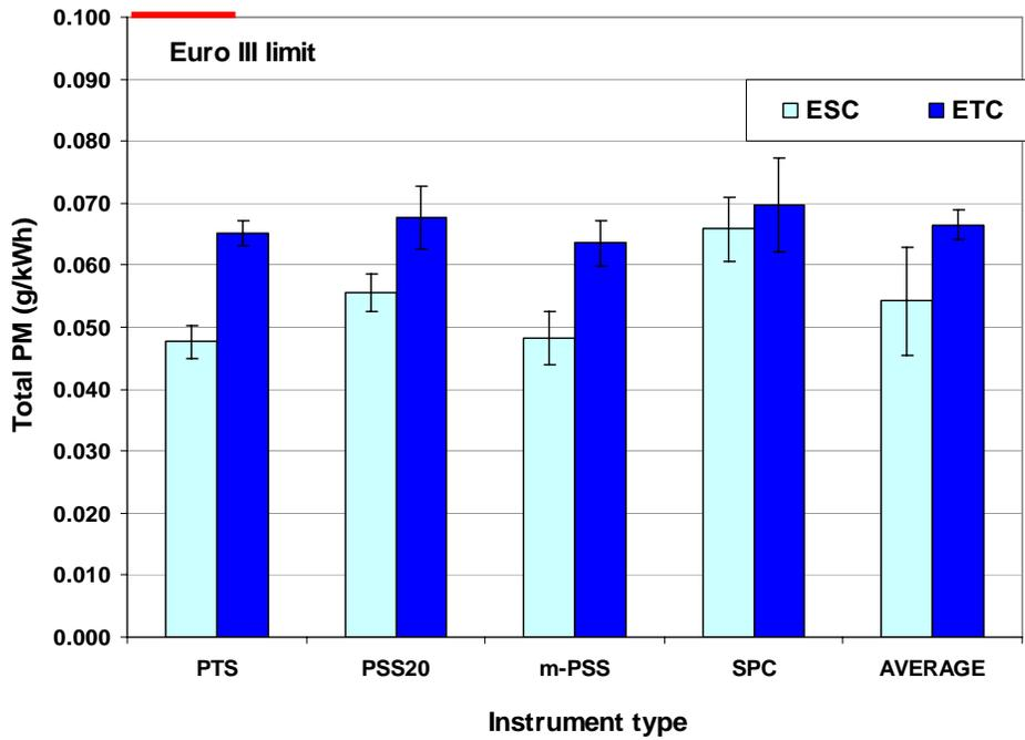
**Figure 3:** Comparison of PM mass laboratory measurements among different PM instruments over both ETC and ESC cycle.
