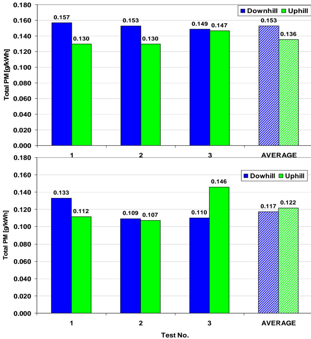
**Figure 11:** City bus PM data: Total PM mass (g/kWh) collected on filters using the Control Sistem m-PSS over three consecutive tests over line 17 and 74 distinguishing between one-way (downhill) and return (uphill); average values are reported as well.
