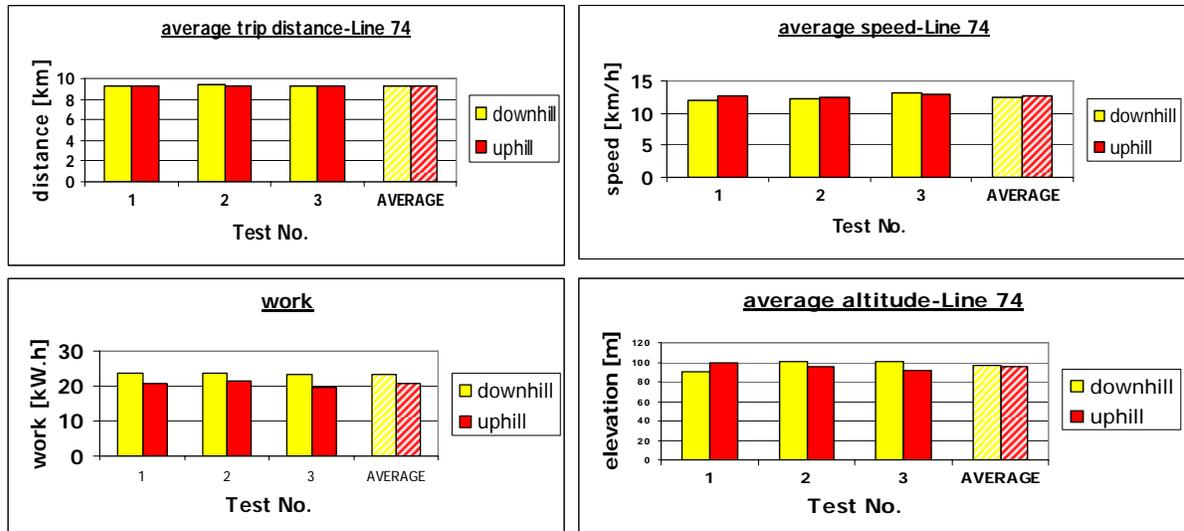
**Figure 9:** City bus test trip characteristics: trip distance, average engine speed, average engine work, average altitude for line 74.
