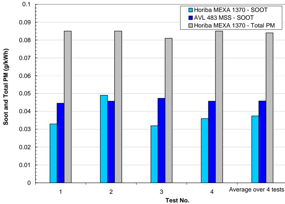
**Figure 7:** Total PM and soot measured with the MEXA1370-PM and the AVL 483 MSS respectively over the ETC cycle, standard diesel fuel.
