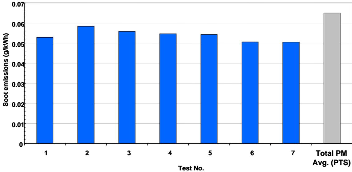
**Figure 5:** AVL 483 MSS total soot measurements (g/kWh) over 7 consecutive ETC tests; the average PM mass collected on the filter with the standard method is reported for comparison (full dilution).
