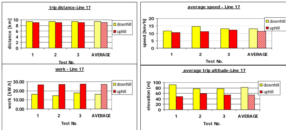
**Figure 8:** City bus test trip characteristics: trip distance, average engine speed, average engine work, average altitude for line 17.
