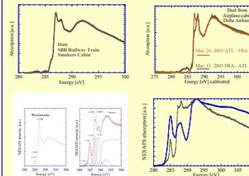
Right: NIST SRM reference materials Spectra of urban particulate matter SRM 1648 (solid, black) and diesel exhaust SRM 1650.
