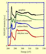
Left: Comparison of spectra from graphite, diesel exhaust, carbon black, and ethylene soot reveals their graphitic nature due to the aromatic setting of carbon atoms in double bonds: C=C. The corresponding  $\pi$  resonance is found at 285 eV. The plateau from 292 to 310 eV is typical for electronically well conducting soot and graphite samples.
