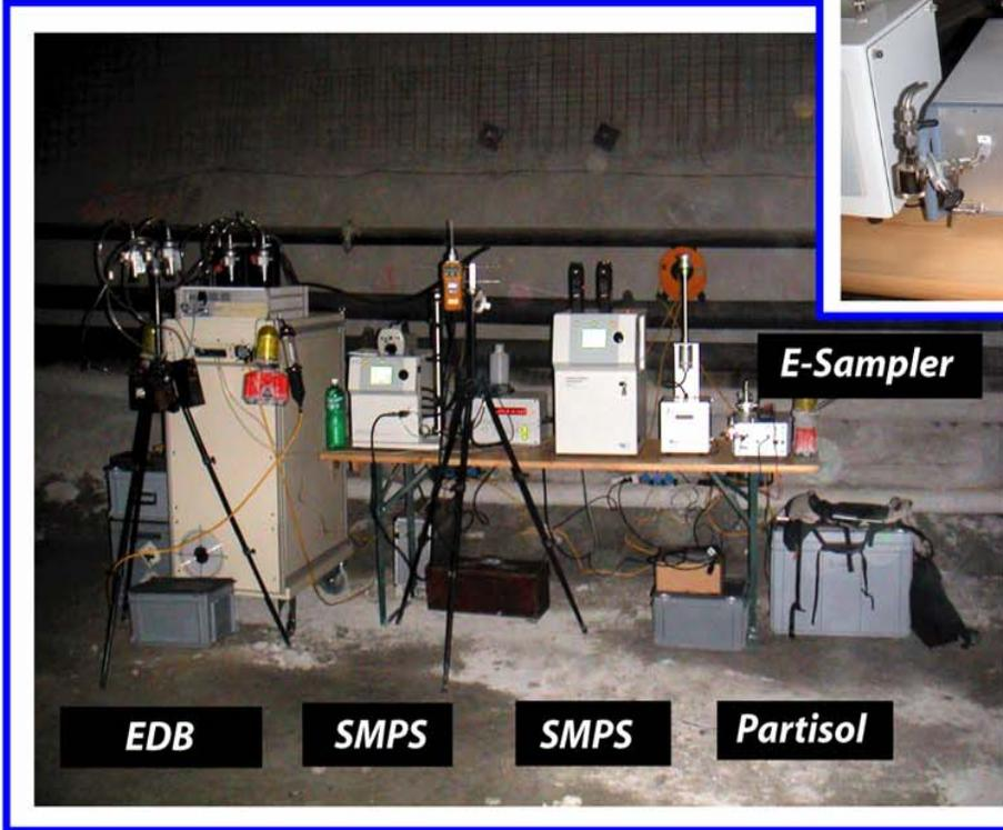
EDB (Electrical diffusion battery) and SMPS (Scanning mobility particle sizer) to measure the particle size distributions on-line.
