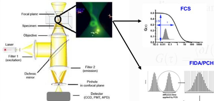
Schematic illustration of the Confocal setup. A laser is fiber coupled with the system. The beam passes a collimator and an excitation filter. The beam is reflected by dichroic mirror and focused into the sample by the tube and objective lens. The emission beam passes again the dichroic mirror and an excitation filter. The pinhole blocks "out of focus" light and the emitted photons are detected by a single-photon-detector (avalanche photon detector -APD).
