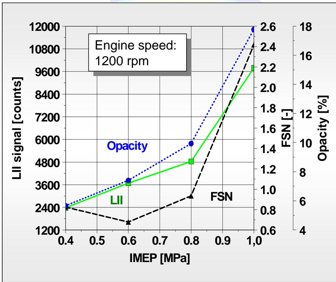
Opacity enables calibration of relative LII signal to obtain absolute soot volume fraction  $f_v$
