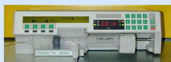
Supply of diluted suspension with Latex spheres to atomizer
