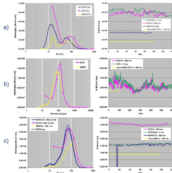
Comparison of ELPI, EEPS and SMPS measurements at static driving speed of Audi
