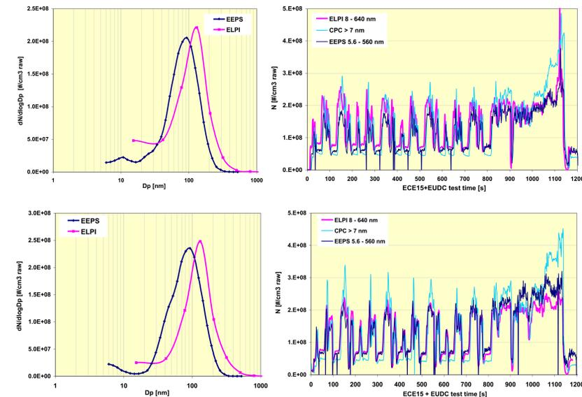
Comparison of ELPI and EEPS measurements in dynamic emission formation conditions. Top: fuel with 1 % lubricant addition (Dr 14x8), bottom: citydiesel fuel (Dr 16x8).
