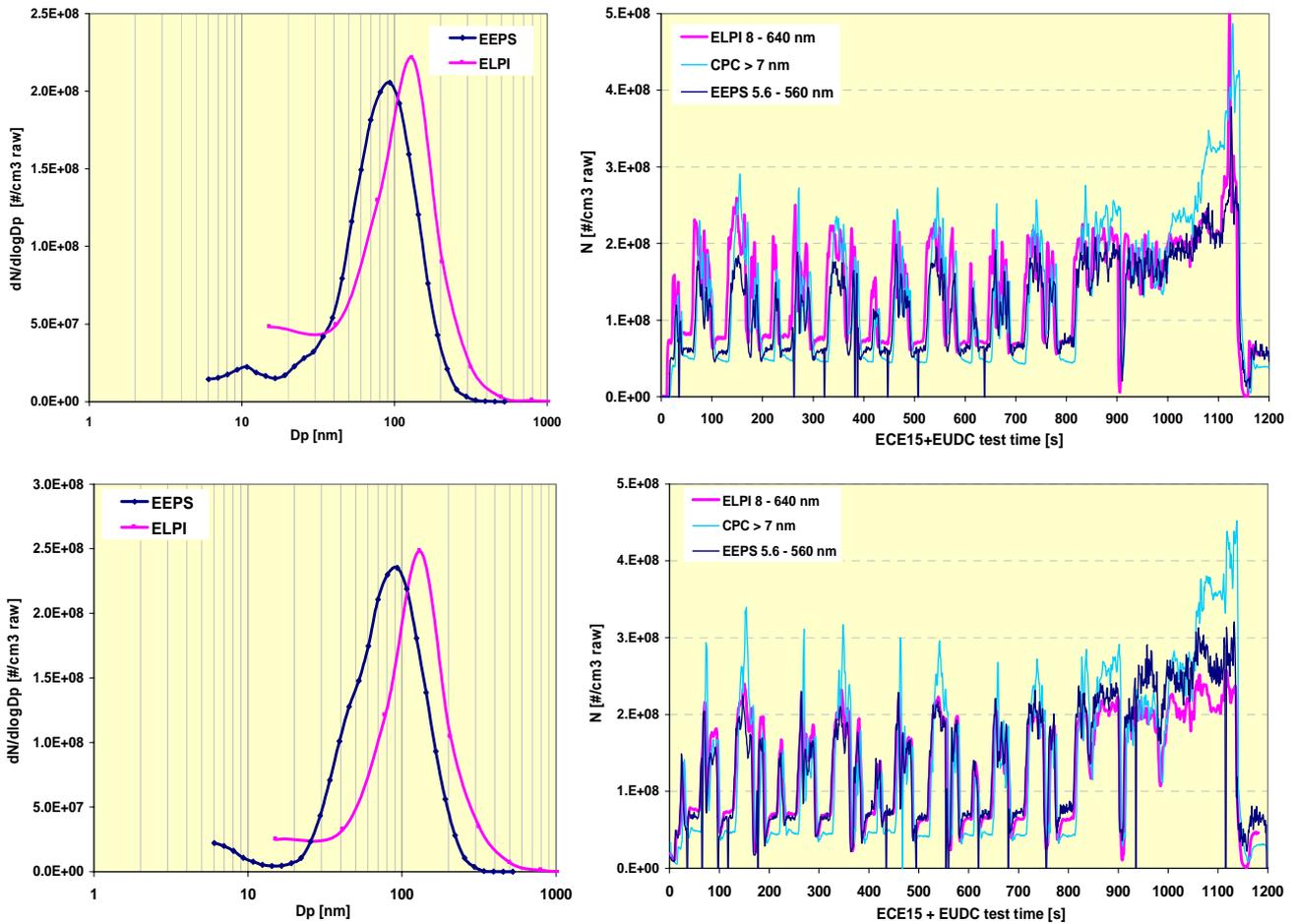
Comparison of ELPI and EEPS measurements in dynamic emission formation conditions. Top: fuel with 1 % lubricant addition (Dr 14x8), bottom: citydiesel fuel (Dr 16x8).
