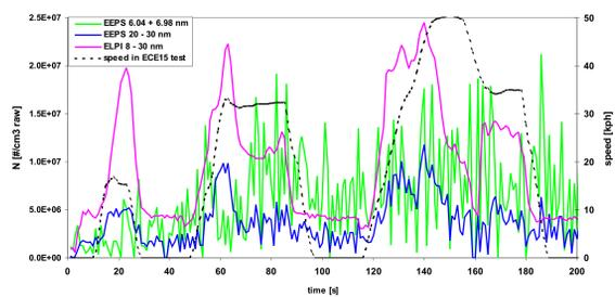
Response of EEPS and ELPI online particle sizing instruments in monitoring nanoparticles in ECE15 test cycle.
