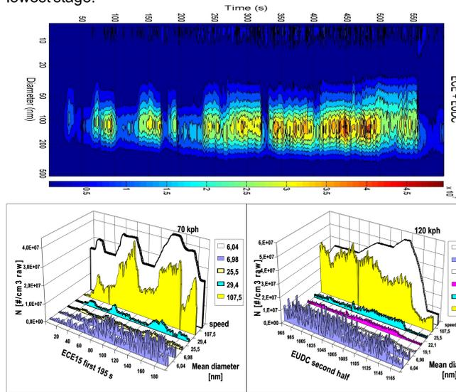
EEPS size spectrum during the first 195 s of ECE15 and at the 50 - 70 - 100 - 120 km/h speeds of EUDC.
