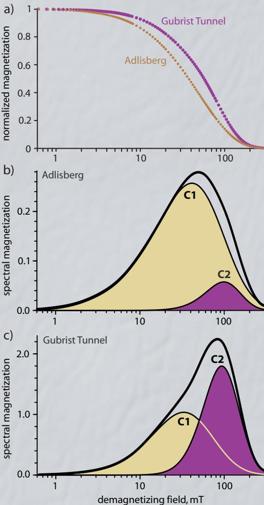
Figure 2. a) Demagnetization of two PM<sub>10</sub> samples from a little polluted site (Adlisberg) and a strongly polluted site (Gubristtunnel). b) Magnetic component C2 is weak at Adlisberg. c) C2 is strong in the tunnel.
