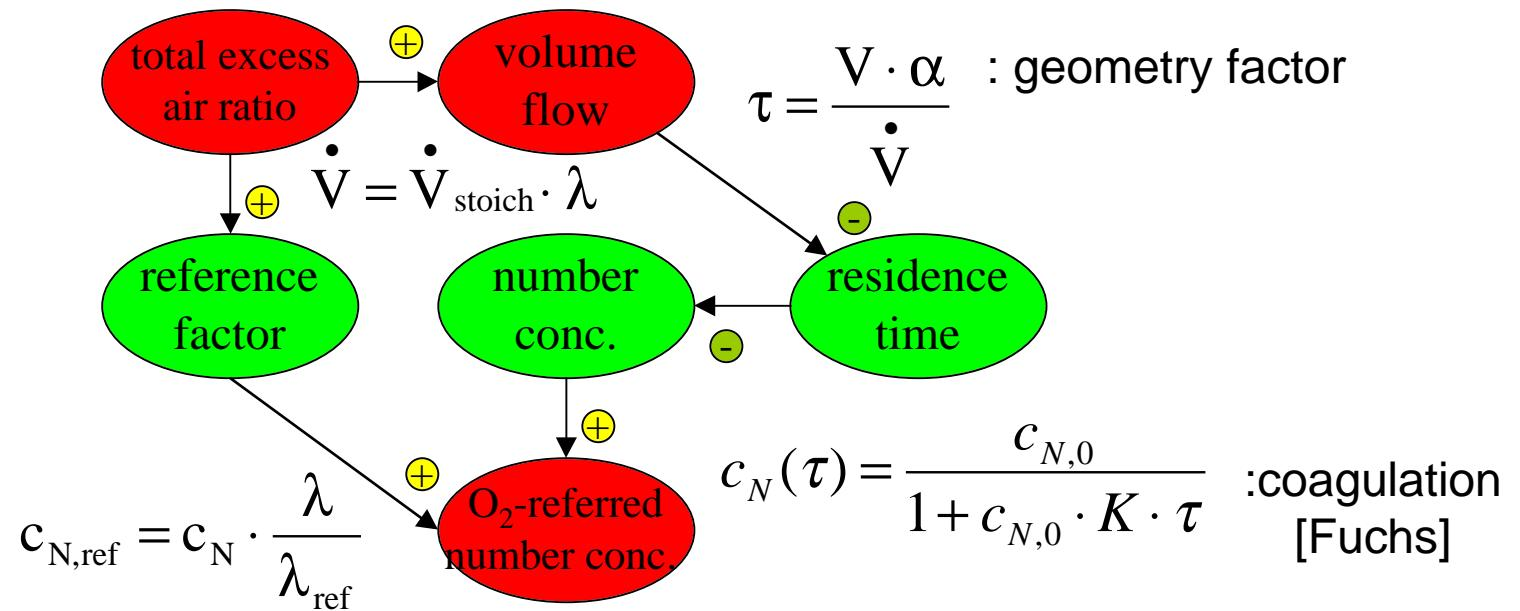
$$c_{N,\text{Norm}}(\dot{V}_N) = \frac{\dot{V}_N \cdot c_{N,0}}{\dot{V}_{\text{NStoich}} \cdot \lambda_{\text{ref}} \cdot \left( 1 + c_{N,0} \cdot K \cdot \alpha \cdot V \cdot \beta_N / \dot{V}_N \right)} = \frac{x \cdot \dot{V}_N^2}{(\dot{V}_N + y)}$$
