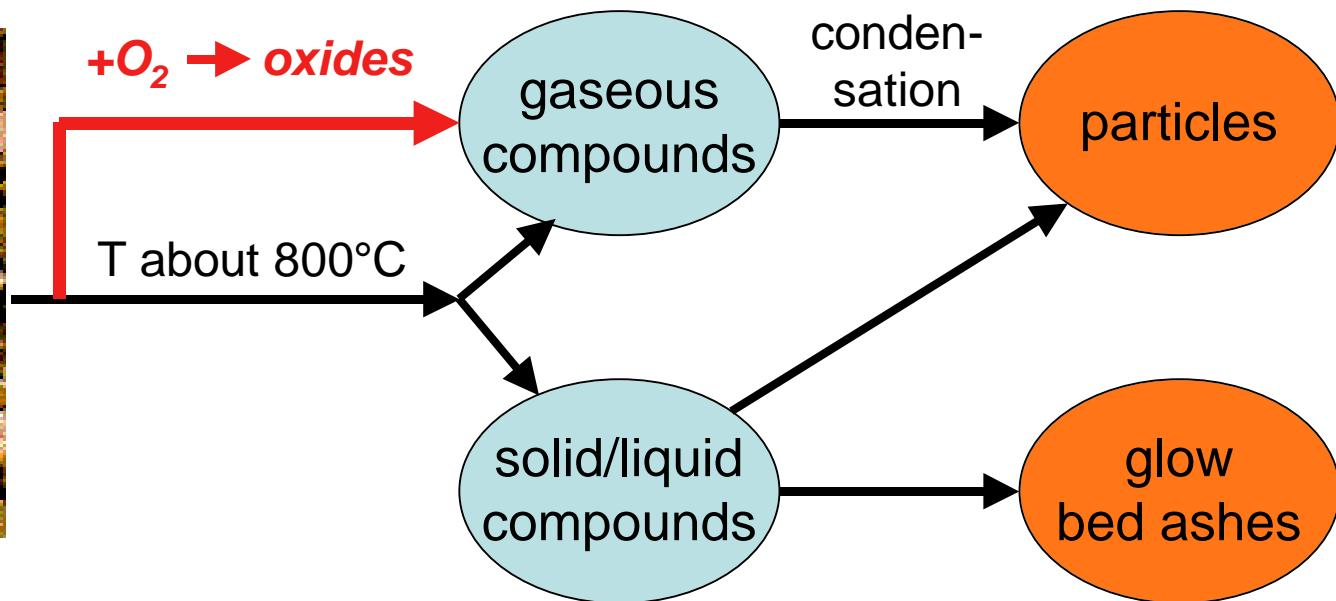
→ Oxygen reduction in the glow bed should cause a smaller potassium load of the flue gas (lower particle mass)
