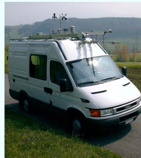
Fig. 1 During YOGAM, a selected route in the Zürich area (left graph) was driven with the PSI mobile pollutant measuring laboratory (right) on a regular base throughout the course of a year, including downtown Zürich (400m a.s.l.), suburban areas (400–500m a.s.l.) as well as rural sites (500– 900m a.s.l.). For the time frame chosen, additional data from official monitoring stations were available for comparison.
