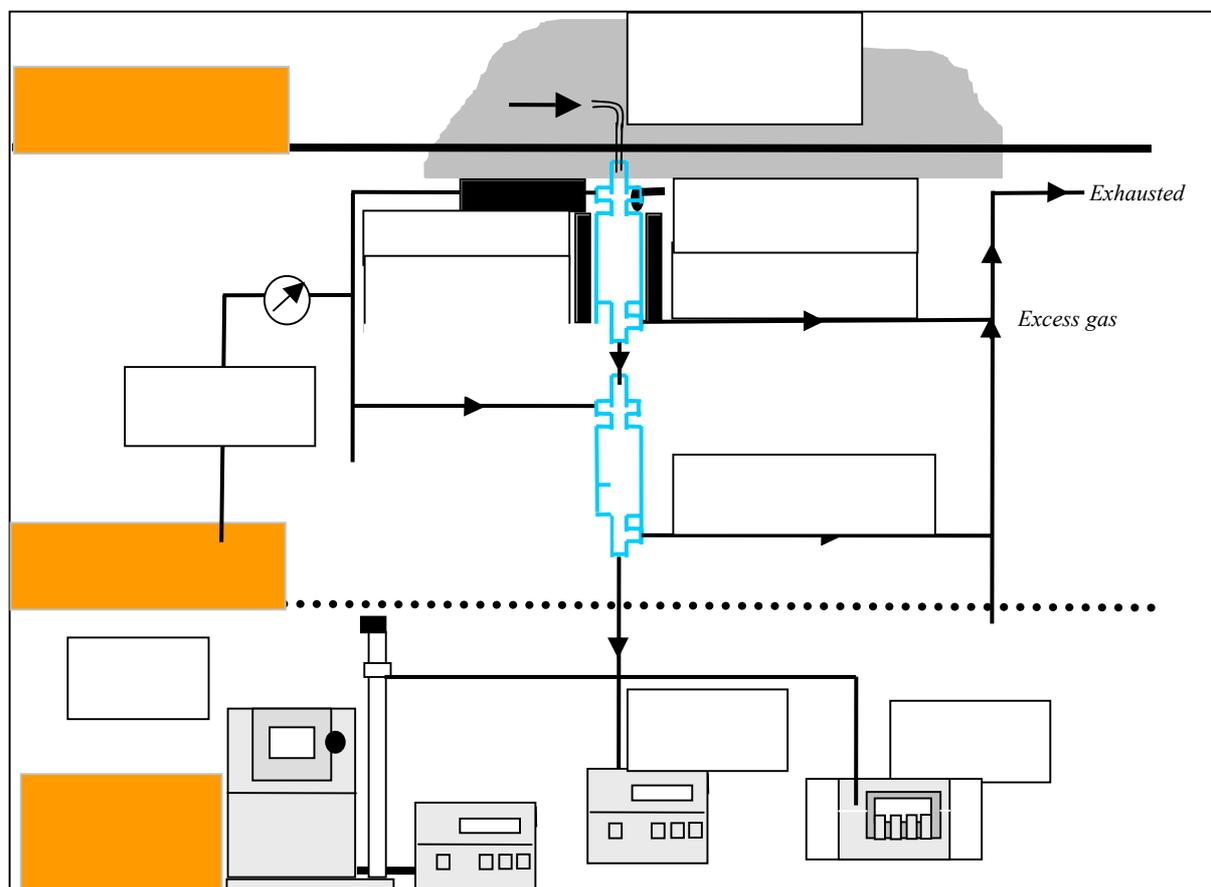
**Figure 7 Two-stage Ejector Dilution System used for PMP Phase 2 testing from engine**
