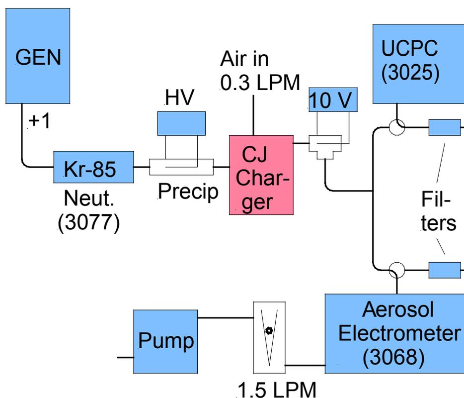
**Figure 4 Instrument for measurement of Mean Charge per Particle of Charger**
