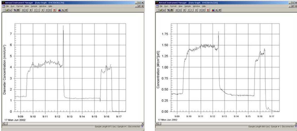
**Figure 8 Instrument Response of EAD (left) and TSI model 3022A CPC (right) at GRPE Particulate Measurement Program Phase 2**
