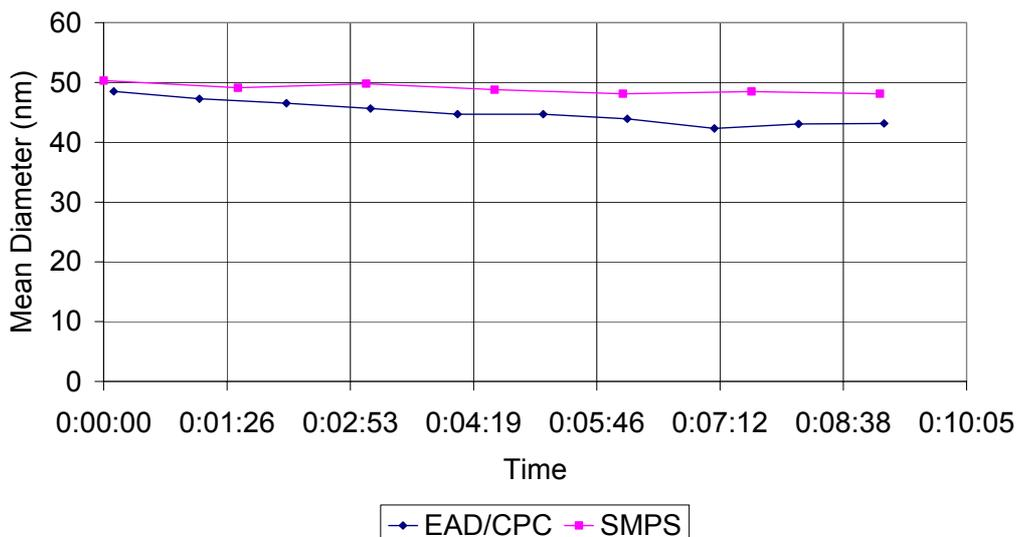
Figure 10 Comparison of EAD/CPC and SMPS Mean Diameters
