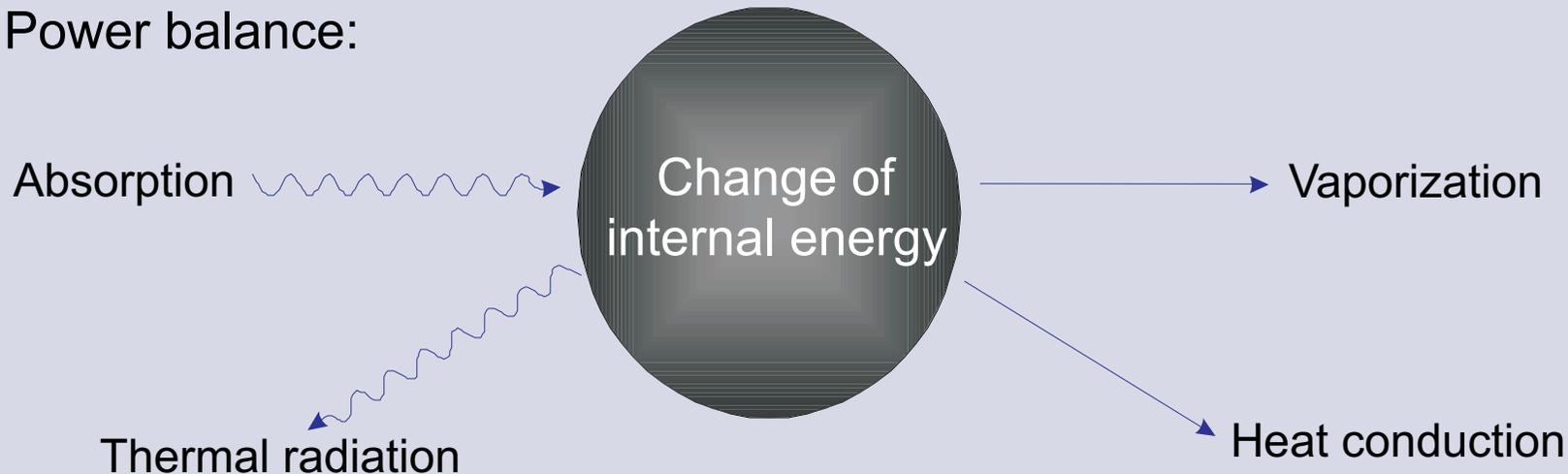
$$\underbrace{Q_{abs} \cdot \frac{\pi d_p^2}{4} \cdot E_i}_{\text{Absorption}} - \underbrace{\Lambda \cdot (T - T_0) \cdot \pi d_p^2}_{\text{Conduction}} + \underbrace{\frac{\Delta H_v}{M} \cdot \frac{dm}{dt}}_{\text{Vaporization}} - \underbrace{\pi d_p^2 \int \epsilon(d_p, \lambda) M_\lambda^b(T, \lambda) d\lambda}_{\text{Thermal radiation}} - \underbrace{\frac{\pi d_p^3}{6} \rho C \frac{dT}{dt}}_{\text{Change of internal energy}} = 0.$$
