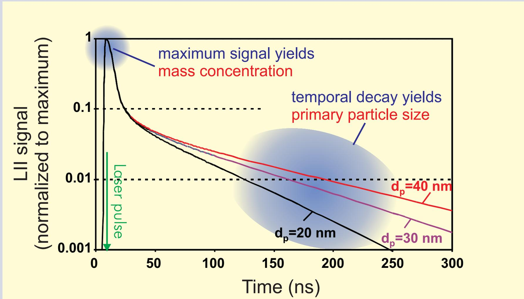
maximum signal in combination with elastic scattering  $\Rightarrow$  aggregate size
