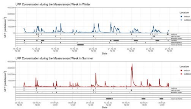
Figure 1: Particle number concentrations over time during summer and winter, with household activities logged below. Figure 2: Distribution of measured indoor and outdoor ultrafine particle number concentrations (PNC) across residential categories during the winter and summer campaign.
