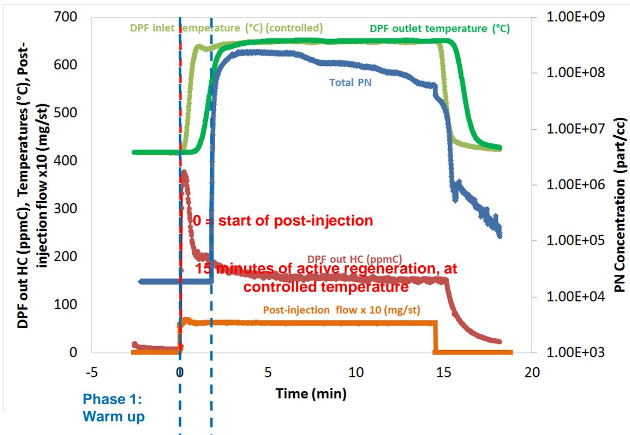
➤ No particulate emissions during the phase 1 despite of the massive HC post-injection
