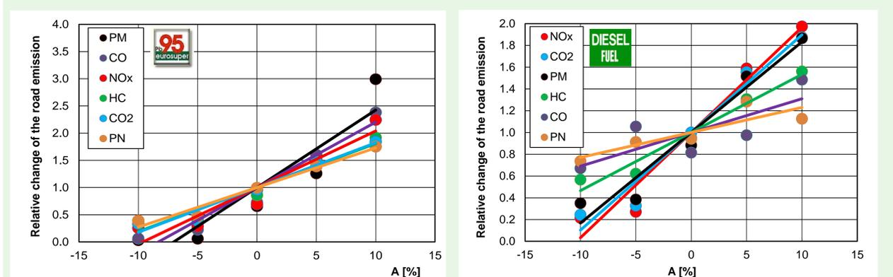
Relative change of the road emission of pollution with the change of the route grade for vehicles fitted with gasoline and Diesel engine
