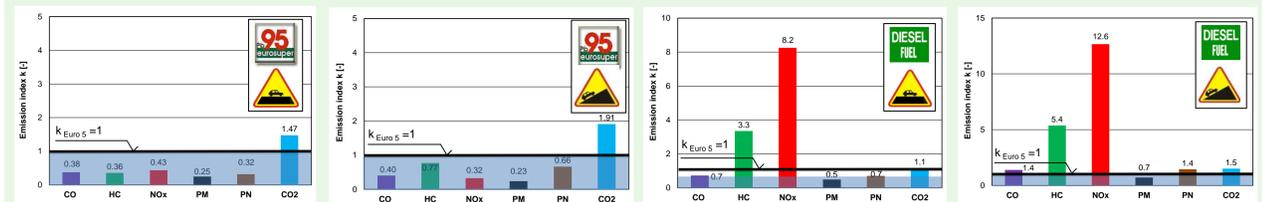
Values of emission factors for vehicles fitted with gasoline and Diesel engine in Euro 5 emission class obtained in emission tests in flat and mountainous terrain
