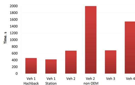
Time to reduce the concentration from 100000 to 4000 UFP per cm<sup>3</sup> for different vehicle types and sizes
