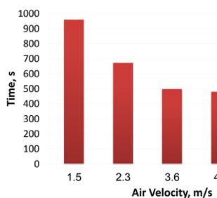
Time to reach 4000 cm<sup>-3</sup> (clean-office value) of UFP concentrations from an initial value of 90000 cm<sup>-3</sup> for various speeds of the air exiting the ventilation channel
