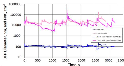
Effects of in-cabin retrofit HEPA filter, inside a shuttle taxi that frequently opens its door for passengers
