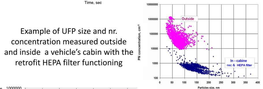
Example of UFP size and nr. concentration measured outside and inside a vehicle's cabin with the retrofit HEPA filter functioning
