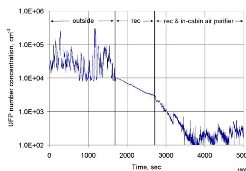
UFP concentration outside and inside the cabin, with AC in recirculating mode and after starting the-retrofit HEPA filter
