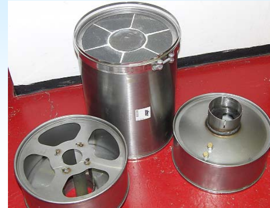
DINEX DiSiC DPF: left –assembled; right – with covers removed
