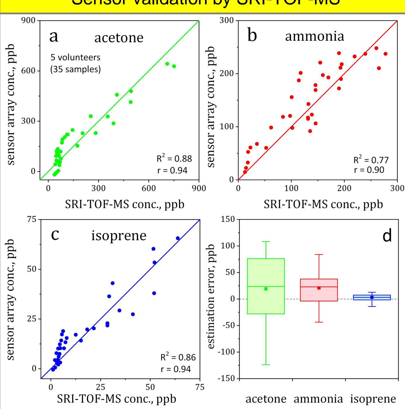
Scatter plots indicating correlations between sensor array and Bench-top SRI-TOF-MS for acetone (a), ammonia (b), and isoprene (c). High Pearson's correlation coefficients (r) and coefficients of determination (R<sup>2</sup>) indicate good agreement between both methods. Box-and whisker plot of sensor array estimation errors (d).
