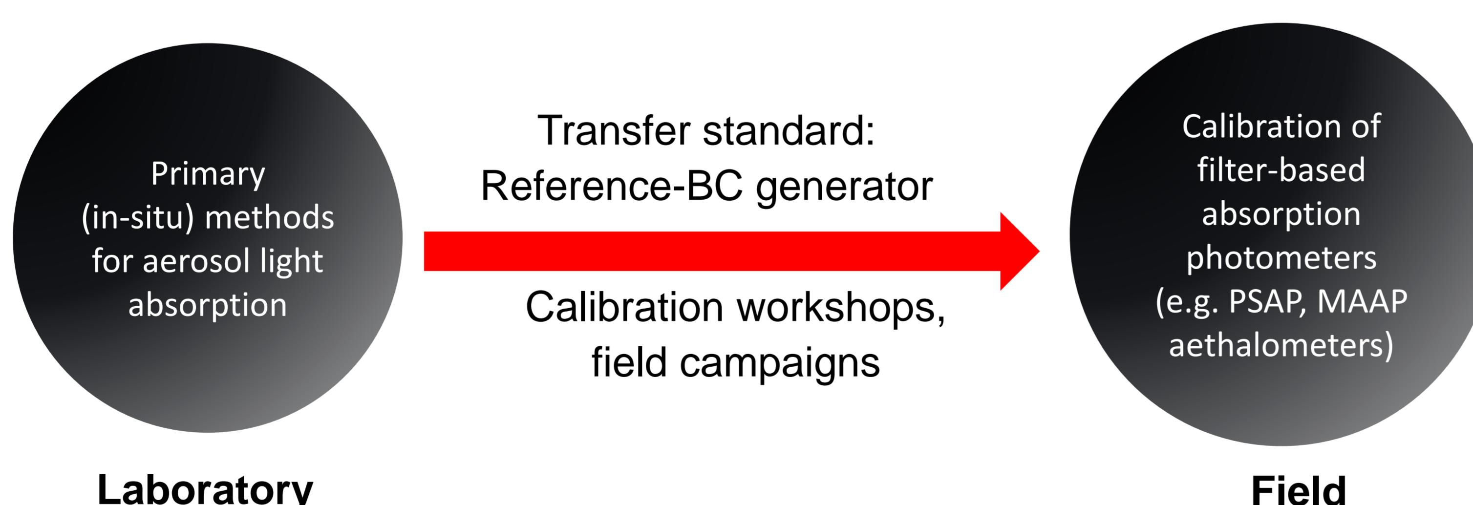
WP3 will build on WPs 1 and 2 to provide a practical and robust calibration procedure for Black Carbon monitoring methods commonly used in Europe<sup>6</sup>. The validation will include checks under controlled laboratory conditions, targeted field campaigns and round robin exercises.
