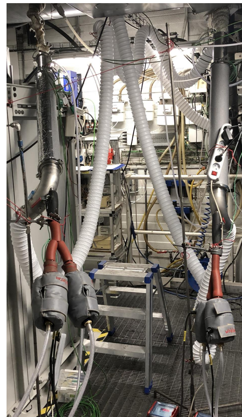
Figure 2. Measurement at MAN Diesel & Turbo's test engine with parallel sampling equipment.
