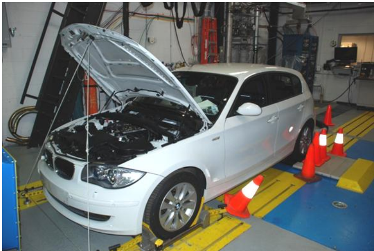
BMW 120i lean gasoline vehicle on chassis dynamometer at ORNL
