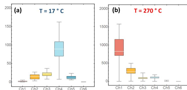
FIGURE 5. Particle size distributions observed for experiments performed at (a.) ambient temperature, and (b.) using heated dilution air
