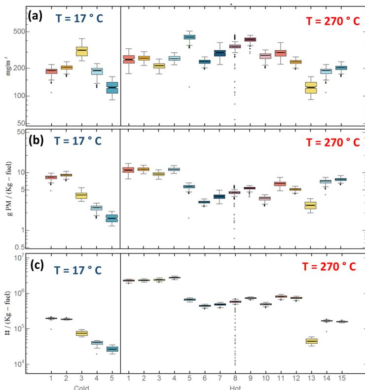
FIGURE 4. Observations for a set of 20 experiments performed during the measurement campaign. The left side is for ambient temperature, and the left side is for measurements with heated dilution air.
