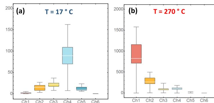
FIGURE 5. Particle size distributions observed for experiments performed at (a.) ambient temperature, and (b.) using heated dilution air
