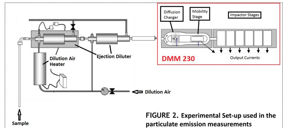
FIGURE 2. Experimental Set-up used in the particulate emission measurements
