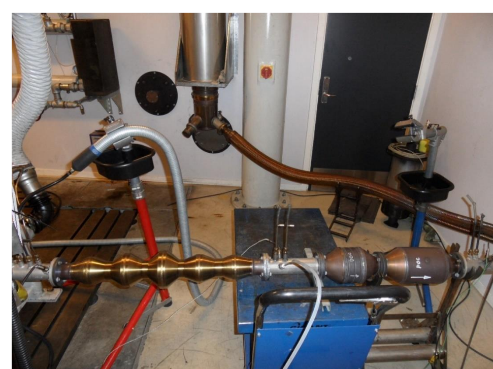
Figure 3. picture of set number 3: Grouping pipe+DOC+POC.
