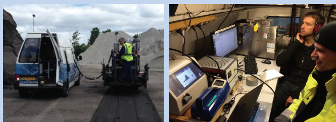
Figures 3 and 4: Experimental setup with measurement equipment inside the van driving next to the selected asphalt paver on a test facility
