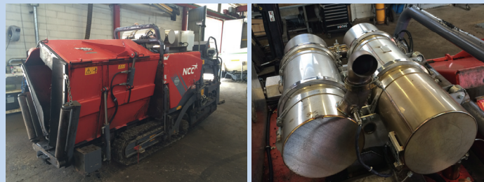
Figures 5 and 6: The asphalt paver with the DPF+SCR solution, developed by Purefi A/S
