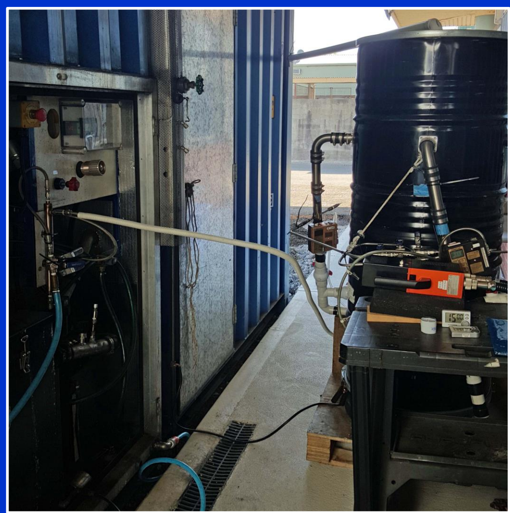
Figure 2 and 3: Experimental Chamber positioned adjacent to engine, respirator filters mounted inside experimental chamber
