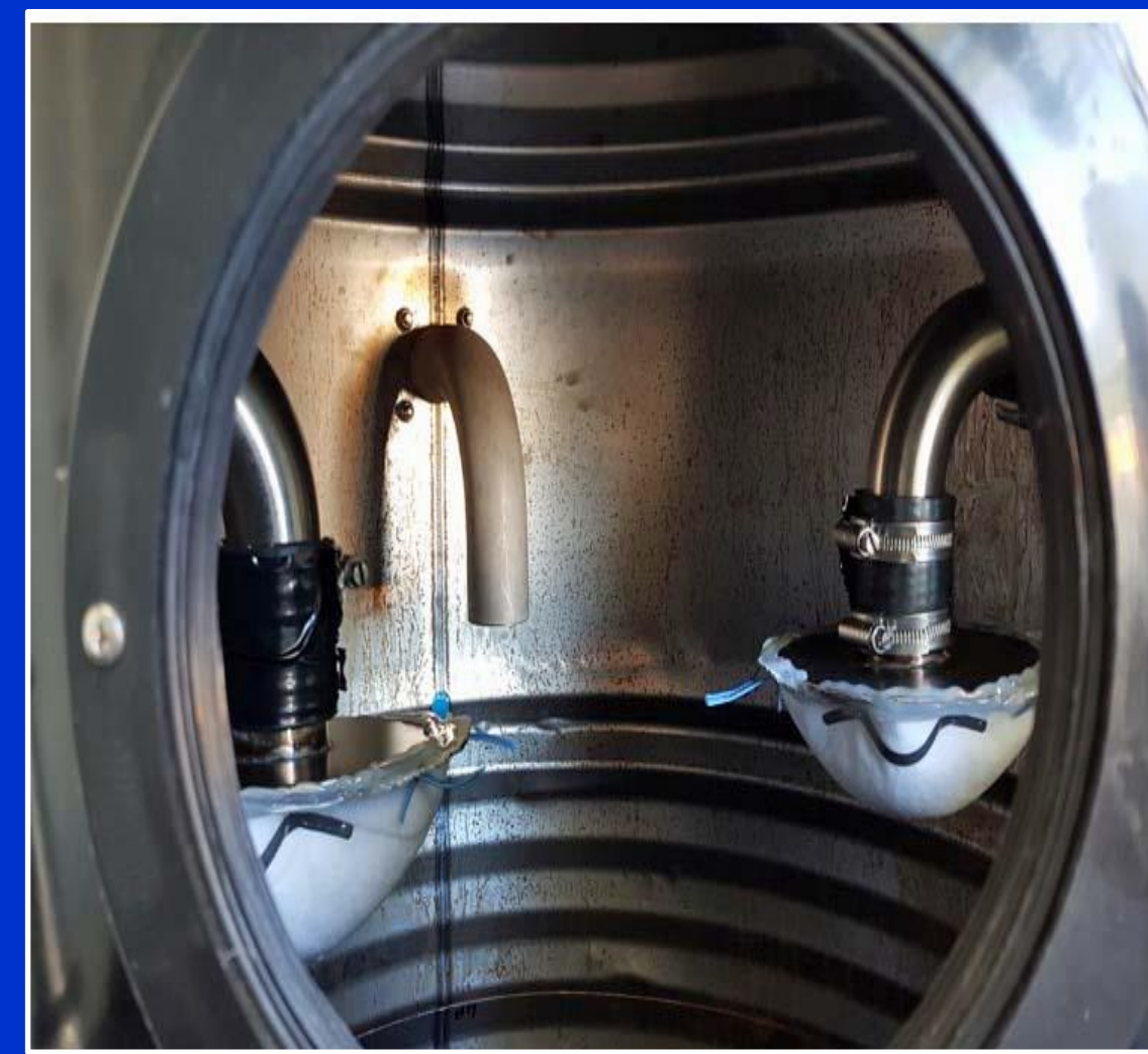
Figure 2 and 3: Experimental Chamber positioned adjacent to engine, respirator filters mounted inside experimental chamber
