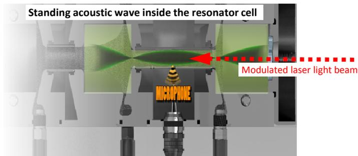
A standing acoustic wave in the resonator is generated by stimulating the particles with a modulated light source.
