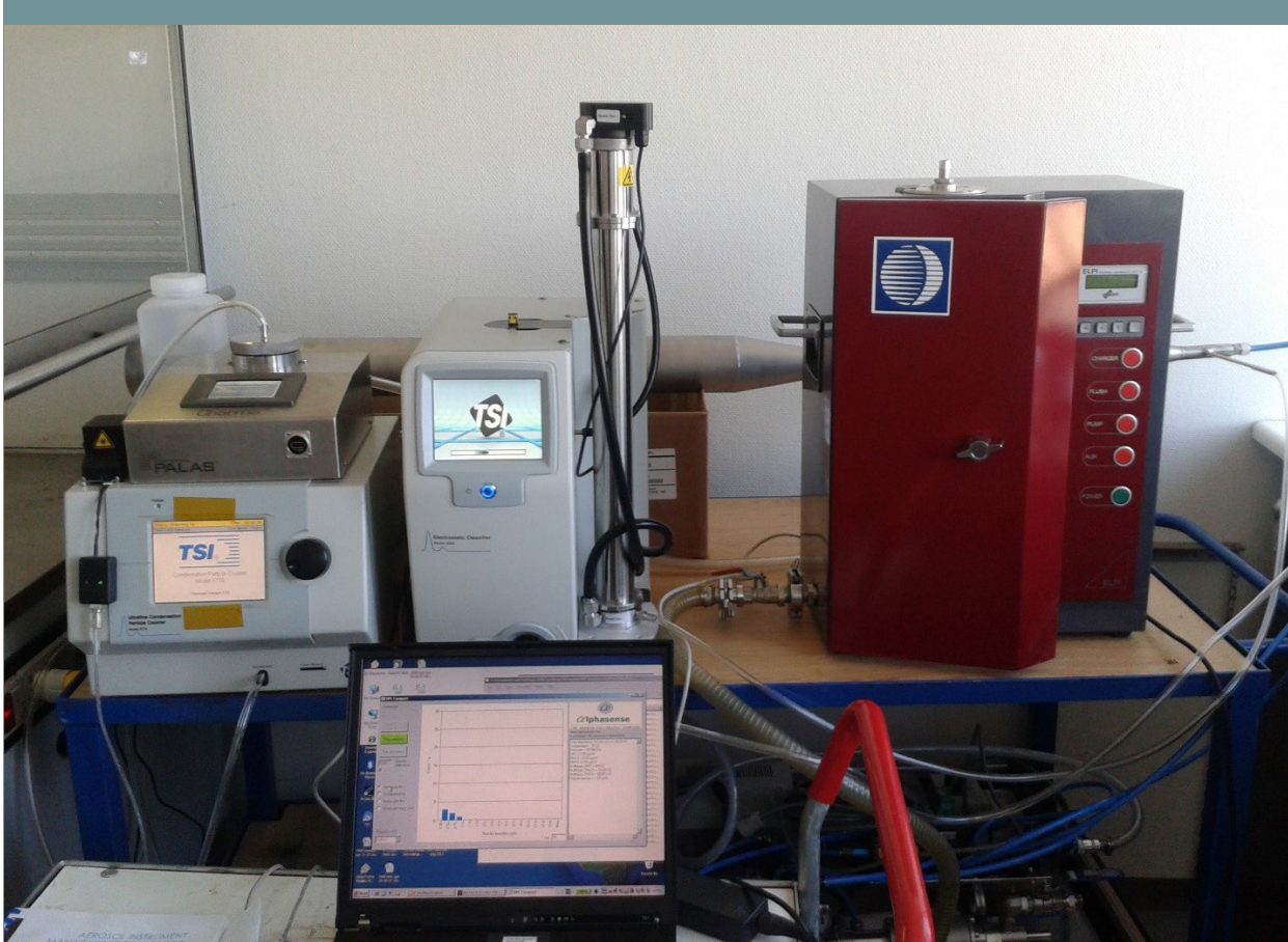
Figure 3. Laboratory setup for testing the Optical Particle Counter using standard particles or sampled air.
