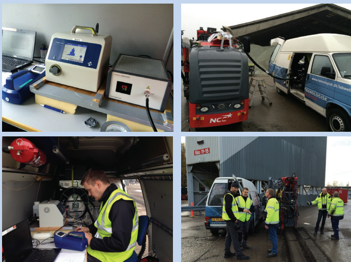
Figure 2: Experimental setup with measurement equipment inside the van driving next to the construction equipment of interest
