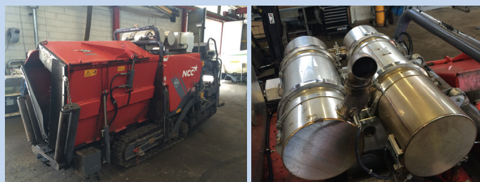
Figure 4: The developed DPF+SCR solution for the asphalt paver.
