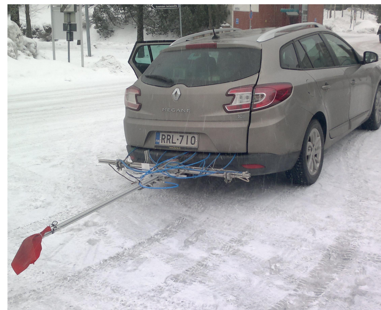
Fig. 1 PEMS installed into a GDI passenger car, a CPC and an EEPS as measuring instruments. The plume sampling is shown on the right hand side.
