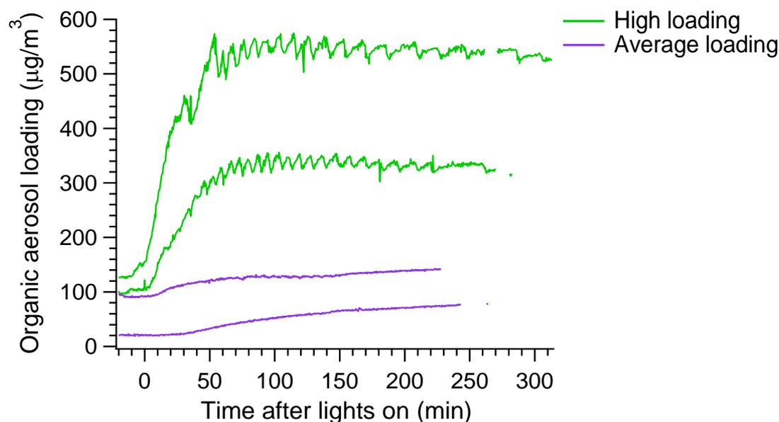
Figure 1. Organic aerosol mass loadings in the chamber as a function of time after UV lights were turned on. High loading corresponds to 7.1-7.8 kg starting wood content in the burner and averaging loading corresponds to 1.9-2.1 kg starting wood content.
