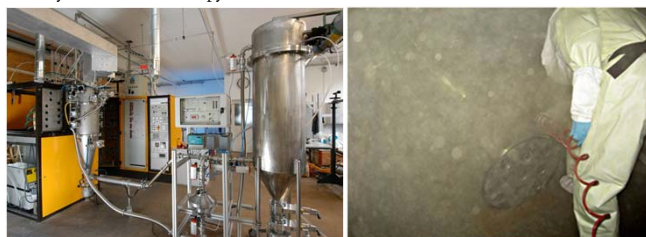
Figure 1. Left: An image of the ICP setup; Right: A photograph demonstrating that the cleaning of the production filter resuspended high concentrations of SiC particles
