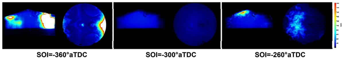
**Fig. 2:** High-speed flame analysis of the injection timing
