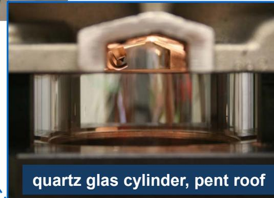
quartz glas cylinder, pent roof
