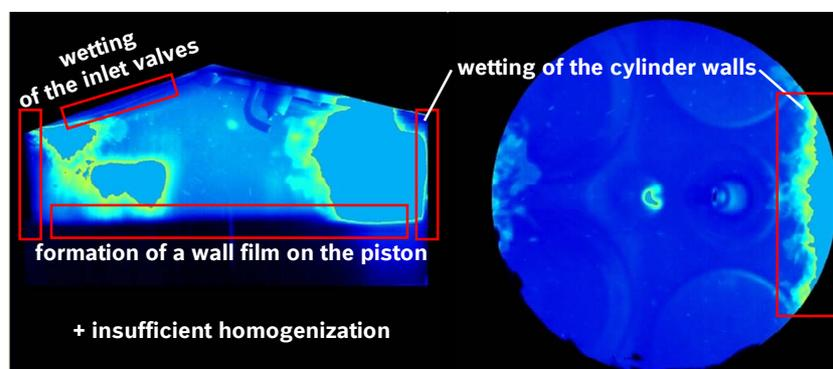
Fig. 1: Typical soot sources which can occur in a gasoline direct injection engine (left: side view in the combustion chamber / right: view from below)
