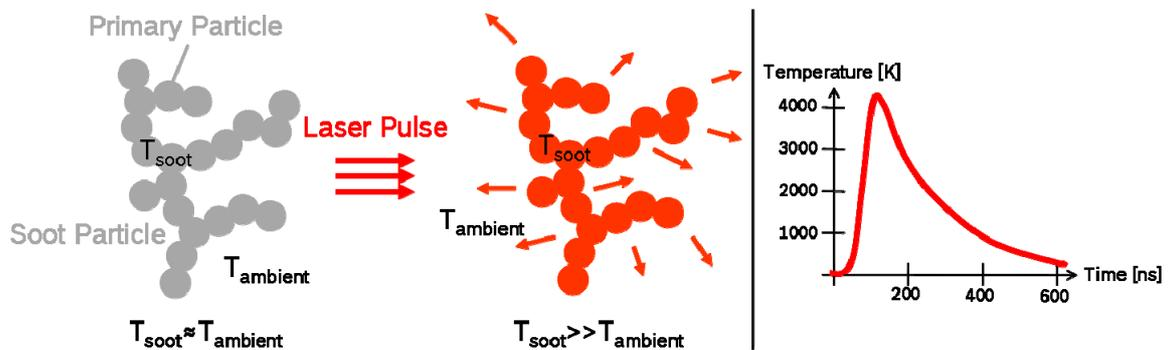
**Fig. 3:** Measurement Principle of the Laser-induced Incandescence (LII)
