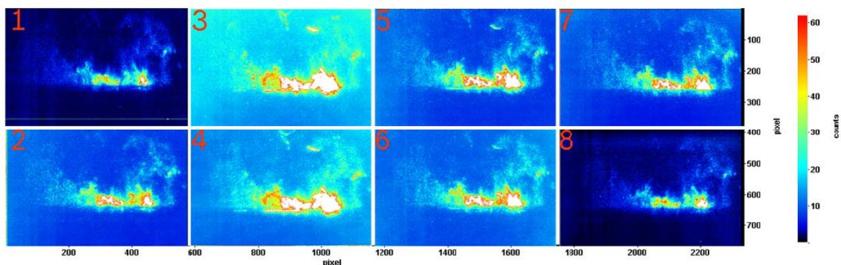
n=2000rpm;  $p_{\text{intake}}=380\text{mbar}$ ; SOI=-19°aTDC; Ignition=-15°aTDC;  $\lambda=1.2$ ;  $T_{\text{Engine}}=20^\circ\text{C}$
