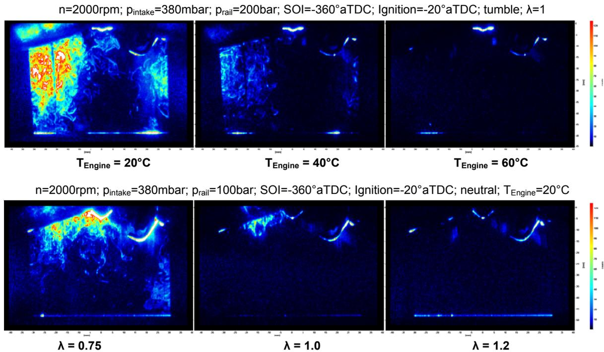
**Fig. 4:** 2D-LII results: Variation of the engine temperature (upper row) and the air/fuel-ratio (lower row)
