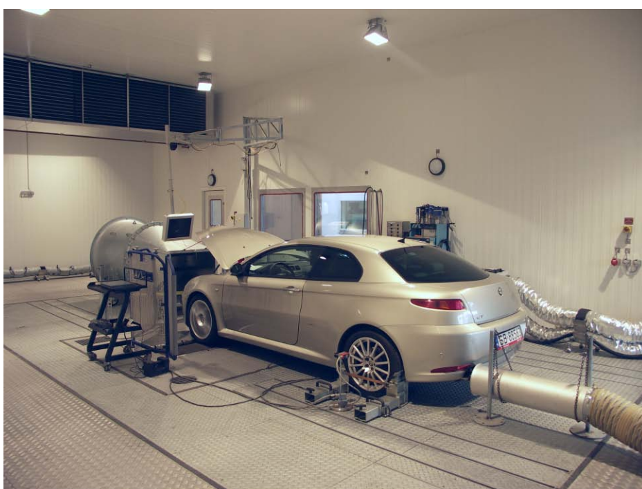
Fig. 1 – BOSMAL's Emission Testing Laboratory – climatic chamber
