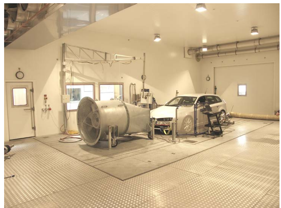
Fig. 2 – BOSMAL's Emission Testing Laboratory – climatic chamber
