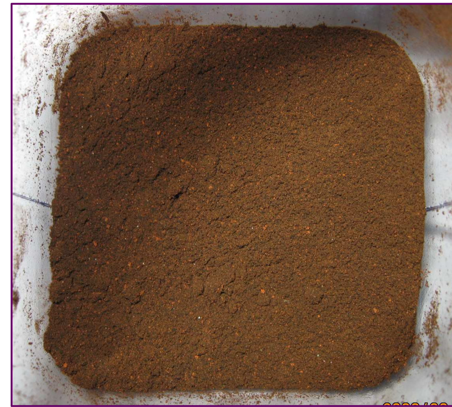
Solid particles removed from DPF after ~500 ml of Satacene consumed with fuel
