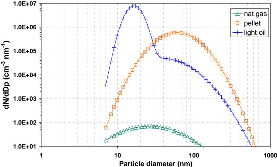
Figure 3: Lognormal distributions fitted to particle size distributions observed during dilution sampling.
