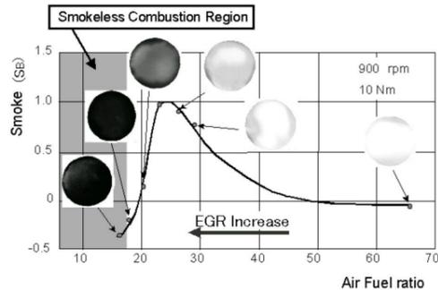
FIGURE 1. REDUCED SMOKE EMISSIONS FROM ADDED EGR.[1]
