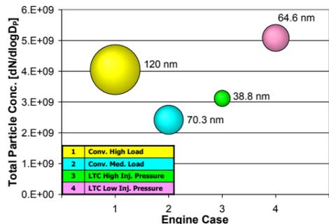
FIGURE 2. VARIATIONS IN PARTICLE SIZE (GEOMETRIC MEAN DIAMETER) AND NUMBER FOR CONVENTIONAL (CASES 1 & 2) AND LOW TEMPERATURE (CASES 3 & 4) DIESEL COMBUSTION.[8]
