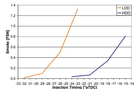
FIGURE 5. SMOKE EMISSIONS FROM BOTH ENGINES FOR ADVANCES IN INJECTION TIMING.
