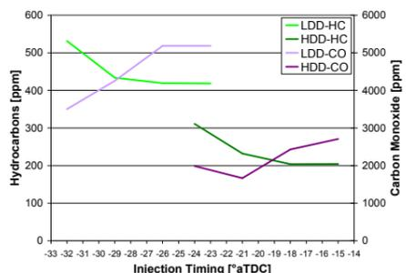
FIGURE 4. HYDROCARBON AND CARBON MONOXIDE EMISSIONS FROM BOTH ENGINES FOR ADVANCES IN INJECTION TIMING.
