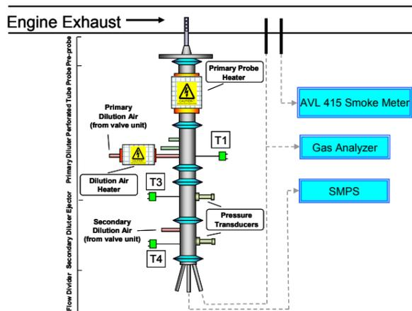
FIGURE 3. LAYOUT OF EXHAUST GAS SAMPLING INSTRUMENTS.
