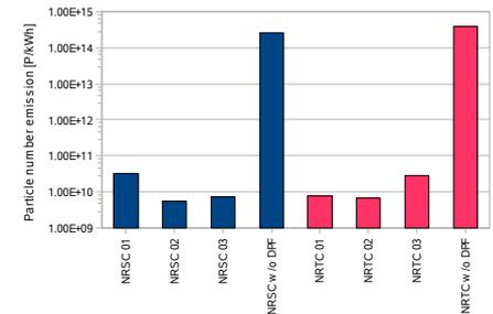
Figure 2. Results of the test cycles with and without particle filter.
