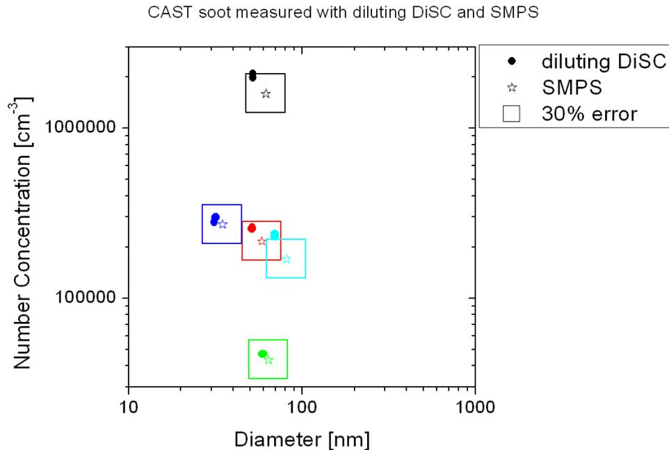
In general, slight overestimation of the particle number and underestimation of diameter likely a calibration issue (calibrated with compact NaCl particles, measured fractal soot particles)
